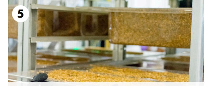
Loose particles are put into a tool where the mycelium grows through and around the particles, forming a solid structure and filling any void space. We let this grow for a few days until it is solid, and then remove it from the tool.
