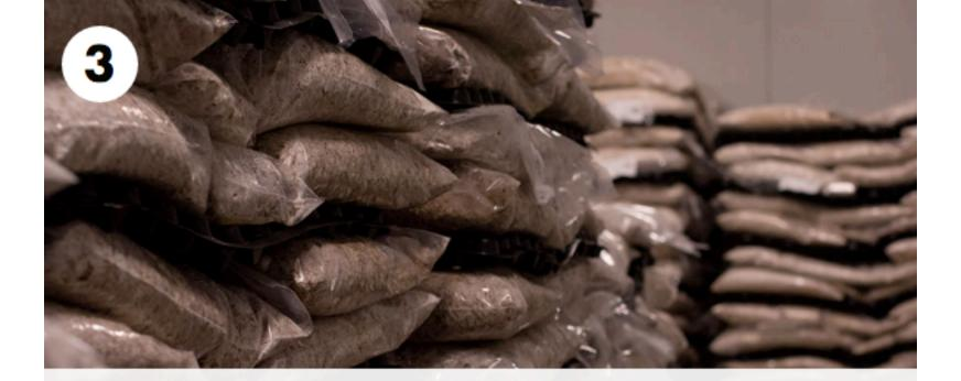
Bag this mixture and let the mycelium grow for a few days. The mycelium sees the agricultural waste as food and reaches out to digest it, forming a matrix of white fibers along the way
